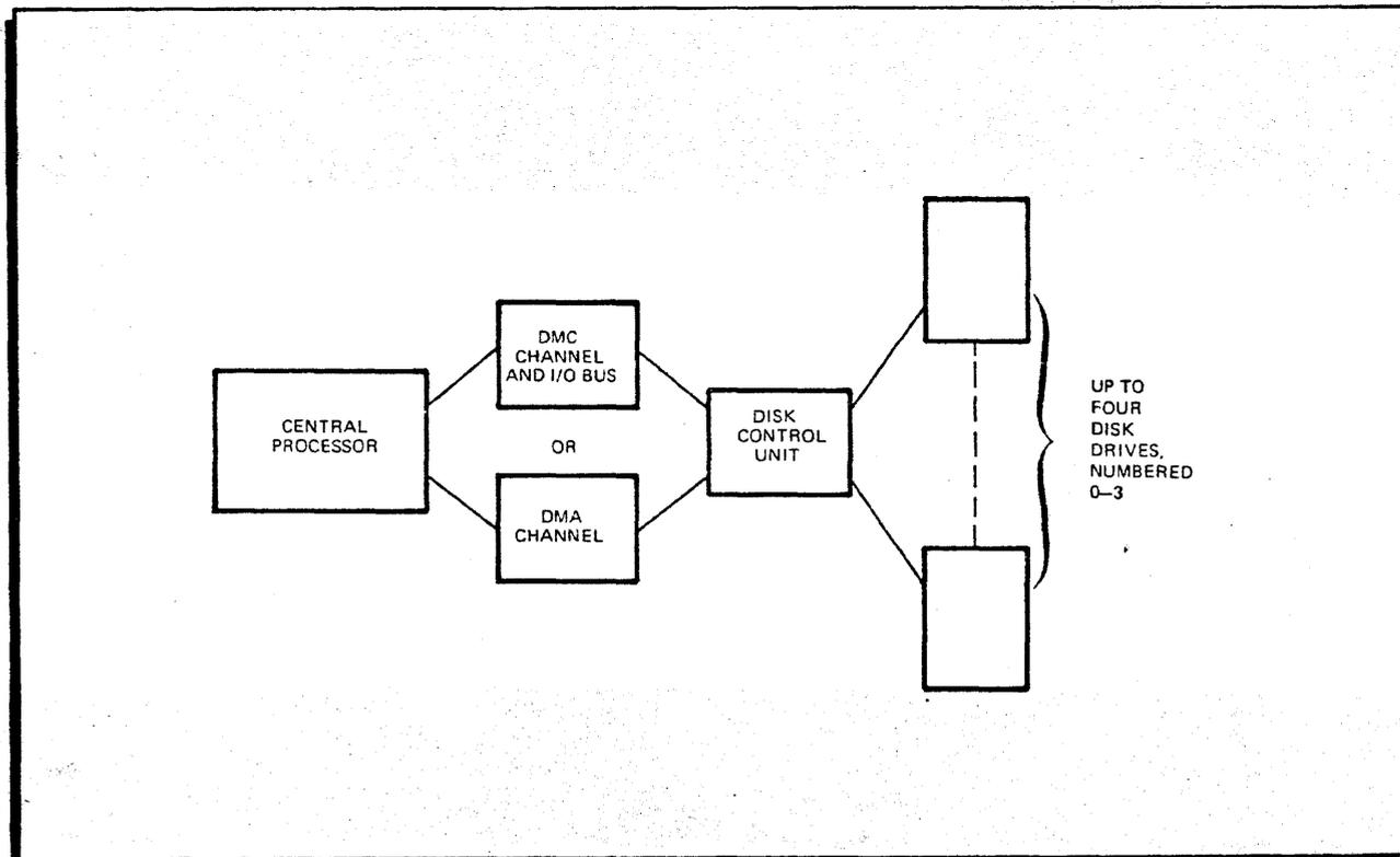
Figure 2-3. Type 4651 System Block Diagram
