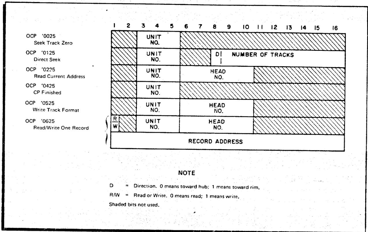
Figure 1-8. 20-Surface Disk Instructions with Required Setup Words
