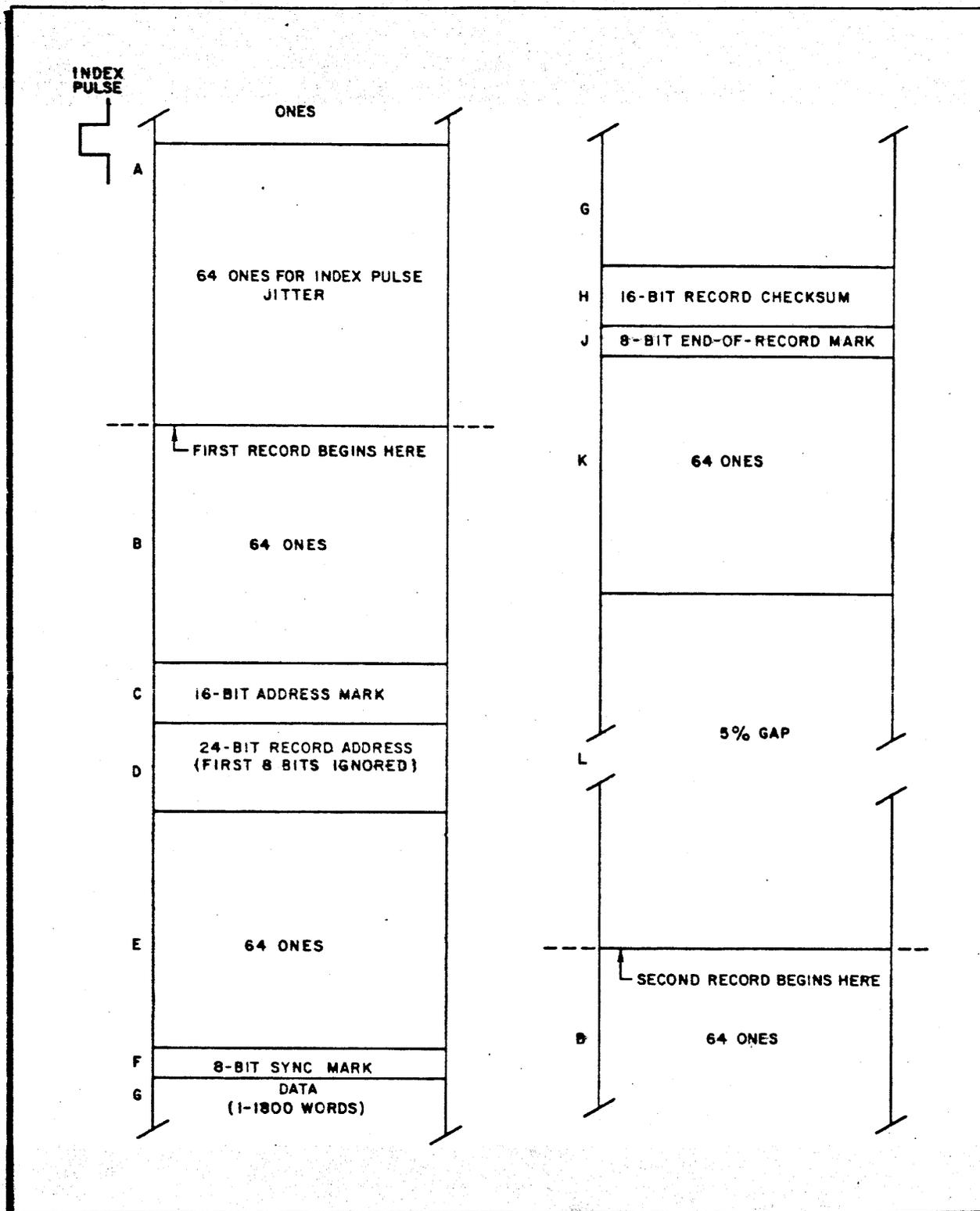
Figure 1-6. 20-Surface Disk Track Format
