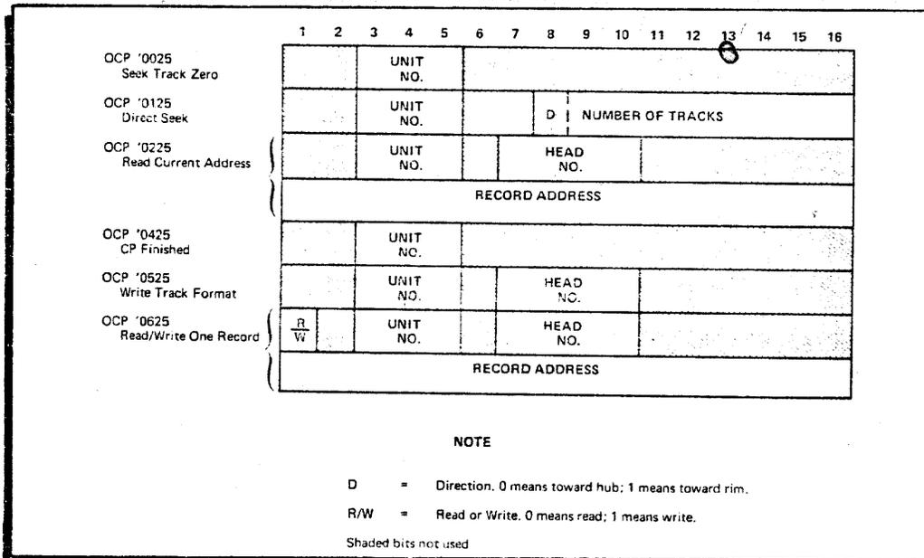
Figure 3-8. 10-Surface Disk Instructions with Required Setup Words
