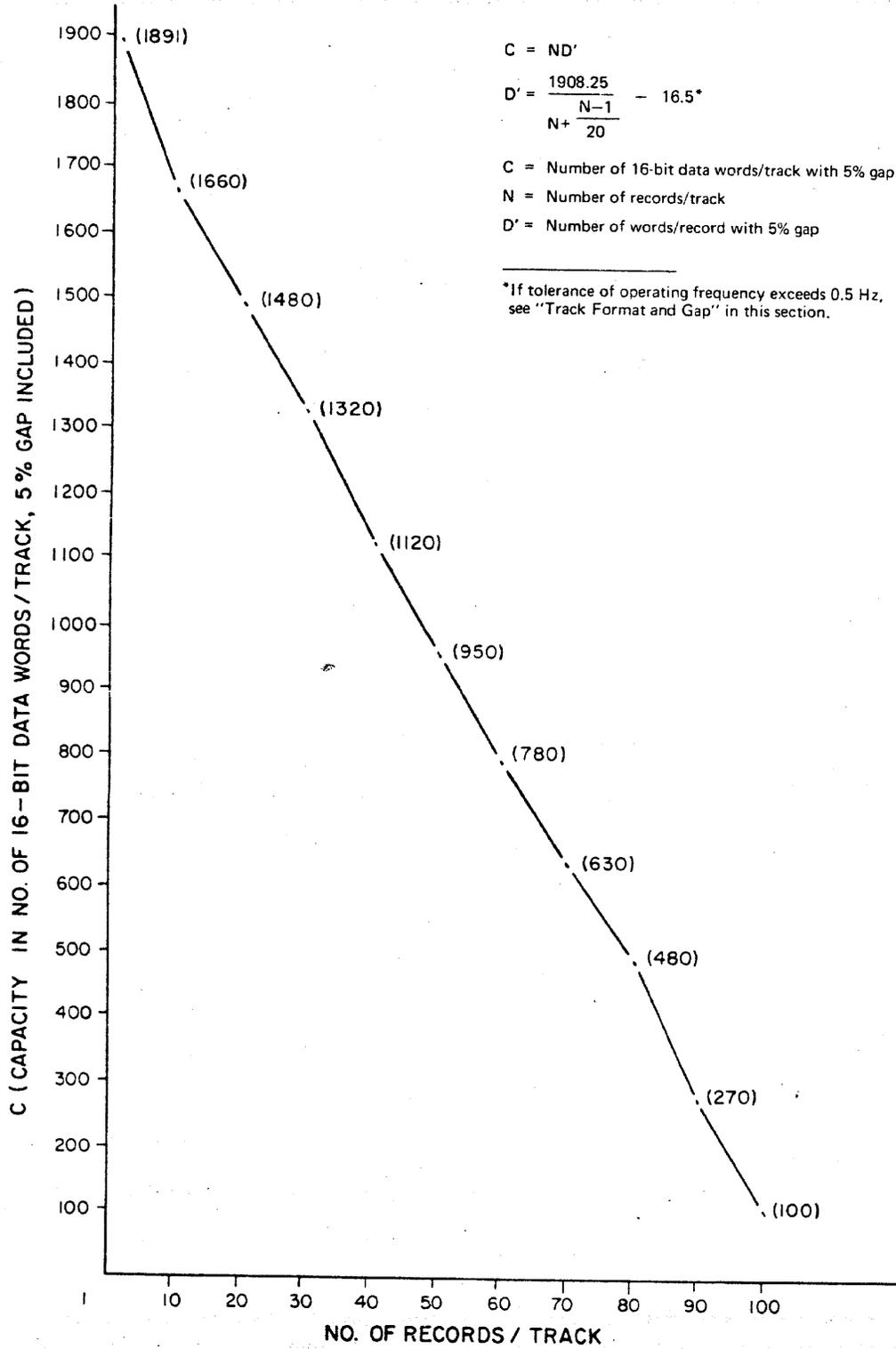
Figure 2-5. 2-Surface Disk Track Capacity vs Number of Records per Track
