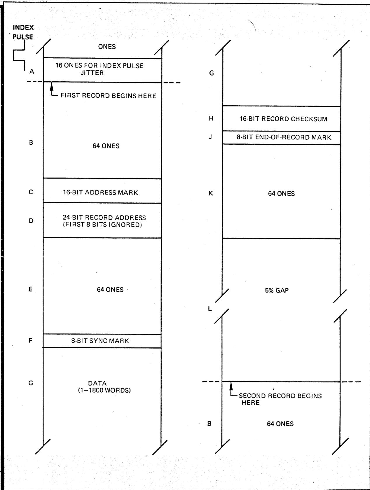
Figure 2-6. 2-Surface Disk Track Format
