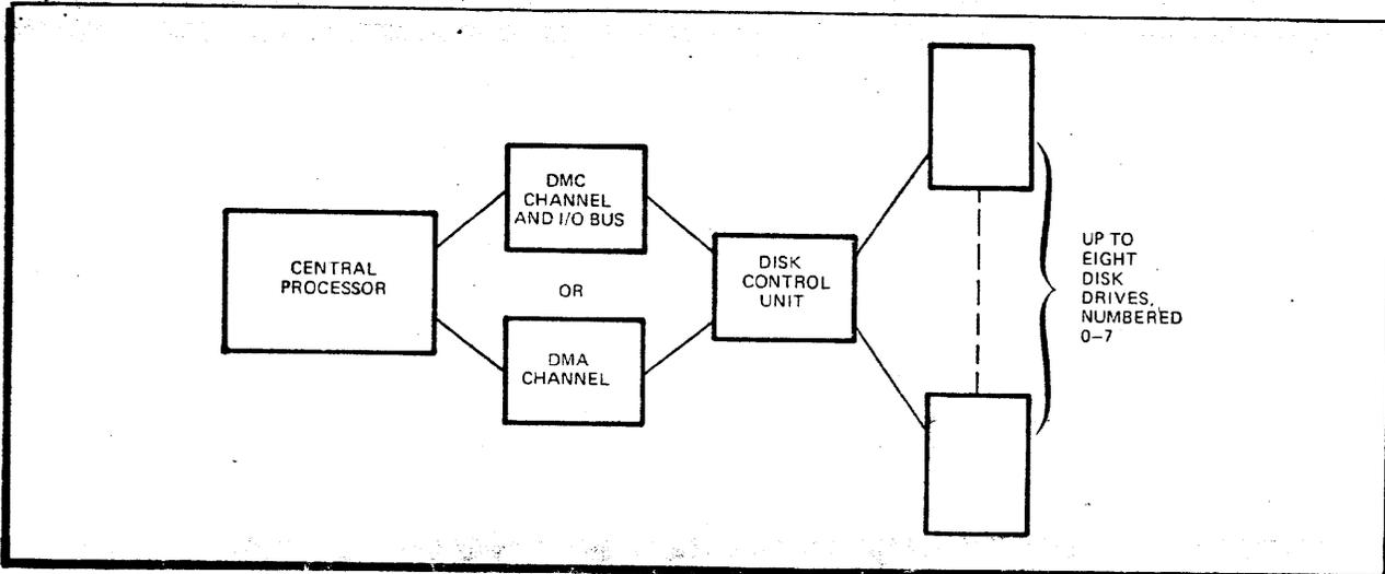
Figure 1-3. Type 4720 System Block Diagram
