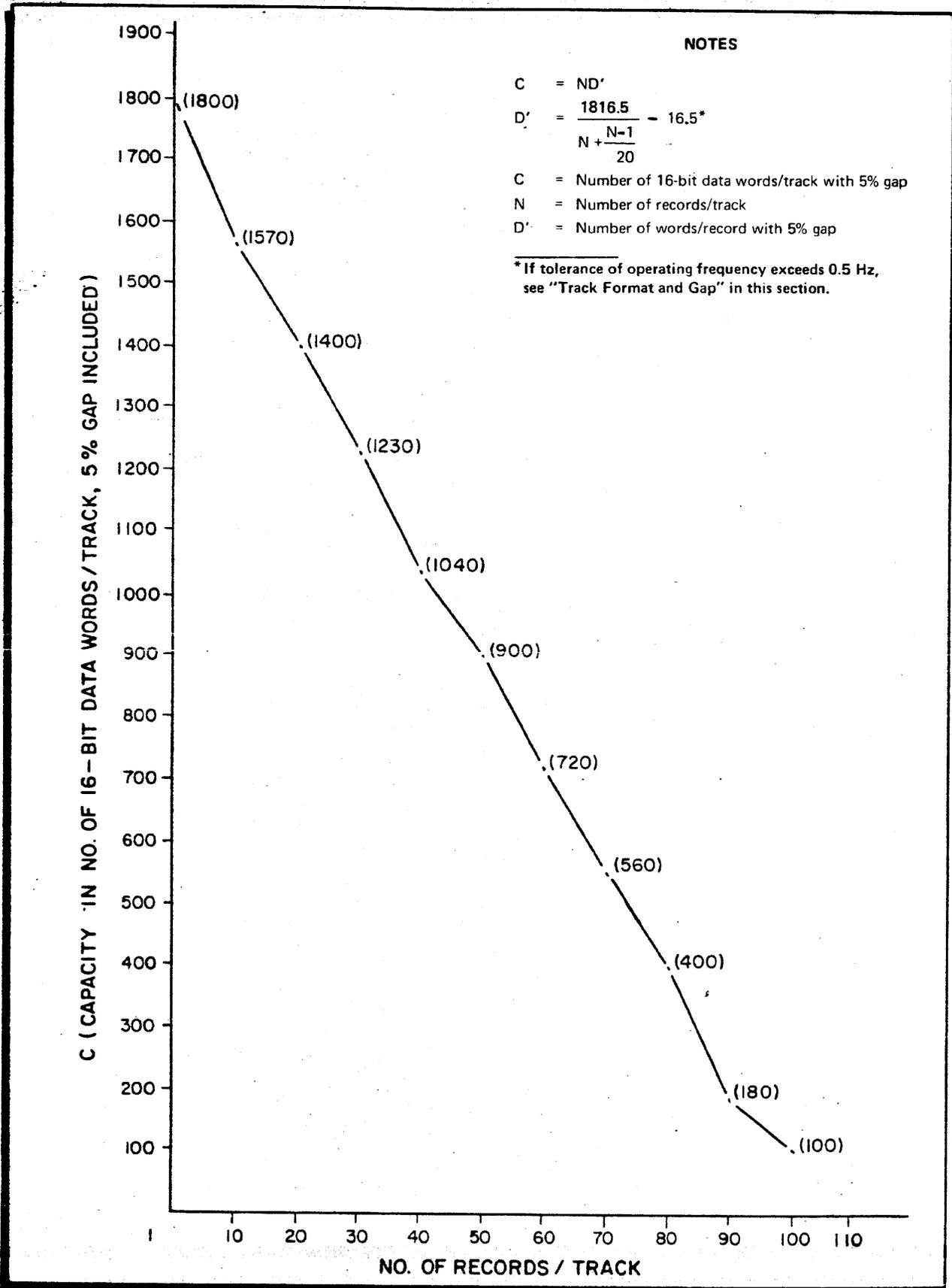
Figure 3-5. 10-Surface Disk Track Capacity vs Number of Records per Track
