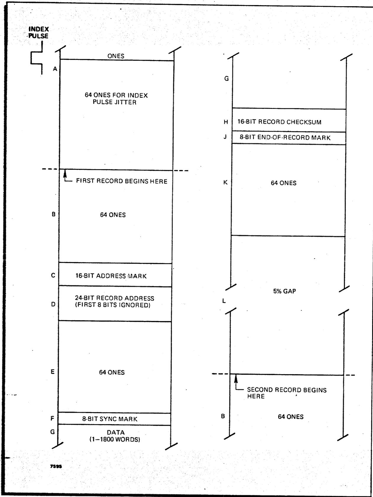
Figure 3-6. 10-Surface Disk Track Format
