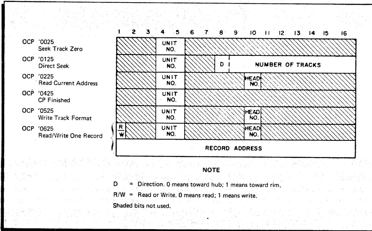
Figure 2-8. 2-Surface Disk Instructions with Required Setup Words
